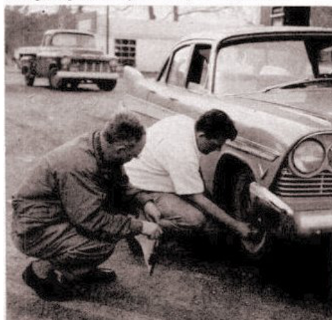
When I took over, I checked the tires . . . and pumped all of them up to 28 pounds.
