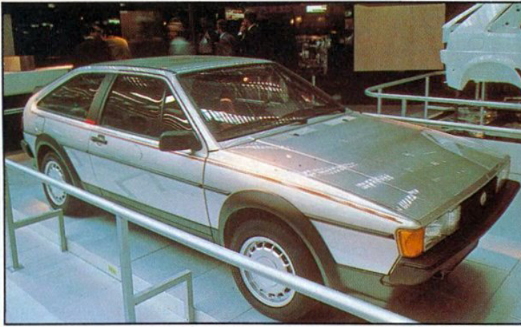
New Scirocco with 16-valve head puts out 102 kW and a strong 160 Nm of torque. Top speed is claimed to be 210 km/h. Car has Bosch mechanical injection, discs all round, stronger driveshafts and low profile tyres on alloy wheels
