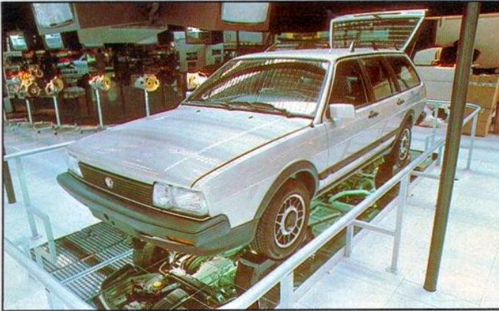
VW Tetra is 4WD Passat wagon with 1994 cm 3 Audi engine and drivetrain and, unlike the Audi, a double wishbone rear suspension. Torque and power outputs are the same as the Audi 80's, but the extra weight reduces performance
