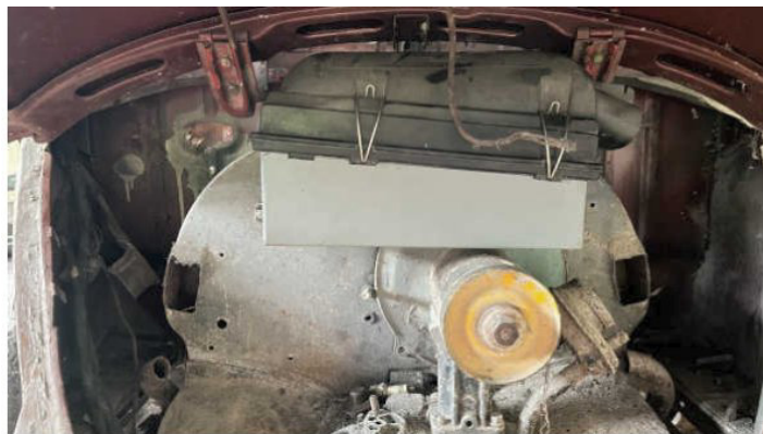
It fits and I can close the engine lid. It needed new brackets to shift it 15 mm to the left and a third bracket to attach it to the AC compressor bolt. There is still room for the front wire hold-down clips to swing.
