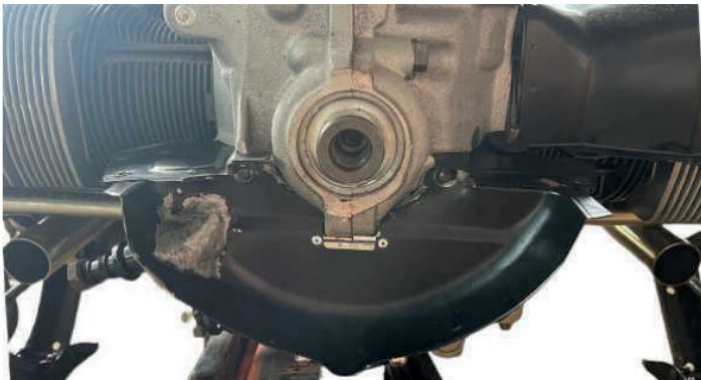
Pulley tin showing panel beating effort around the oil fitting and the patch above the oil pump. If you look really closely, you can make out the rubber grommet around the dipstick tube.
