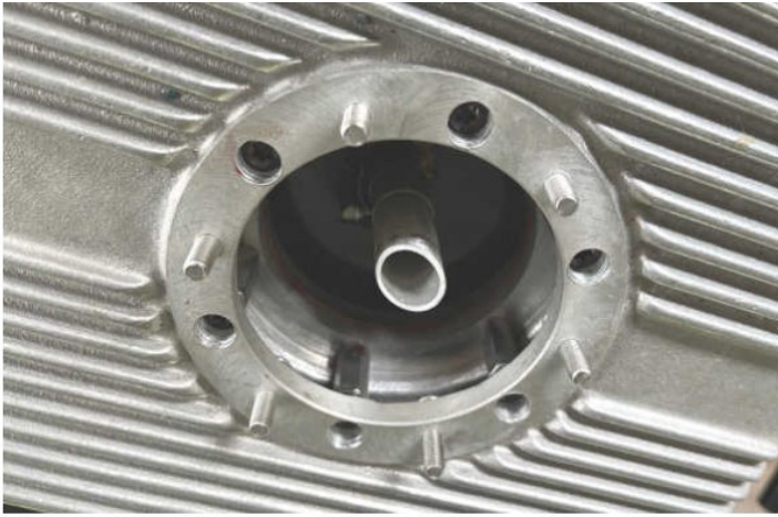
Above the six holes are M6 cap screws which attach to coupling nuts. These screw on to the (longer-than-stock) studs hanging off the bottom of the crankcase. If a coupling nut ever comes loose, it's got nowhere to go.
