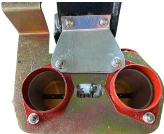
The M5 bolts screw into rivnuts inserted into the fan housing. The velocity-stack stubs are waiting for some mandrel-bent tubing to arrive.
