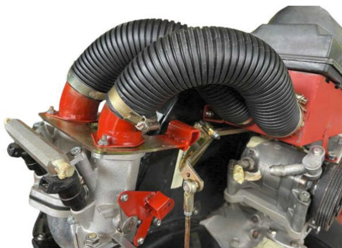
Clearance for the linkage levers is maintained. The extra length between the top of the ITB and the velocity stack inside the air box should shift torque to lower in the rev range, which is fine by me, as the engine will be somewhat rev-limited by the use of hydraulic lifters.
