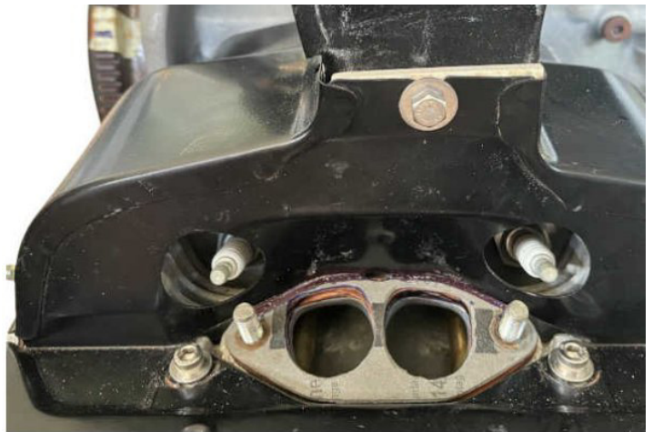
A spacer was needed between the fan housing and cylinder tin, but strangely, only on the left side. It helps to have lots of odd-thickness fibreglass pieces around the shop. Also visible: my modified tin screws.
