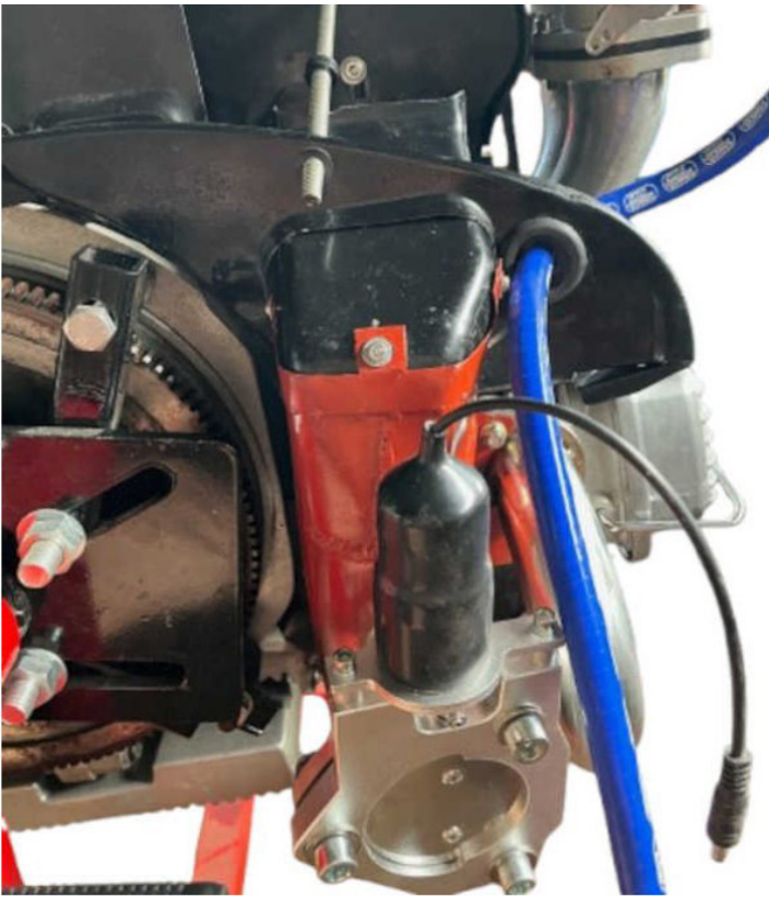
The muffer bypass butterfly valve attached to the oil-cooler outlet duct. Also visible: the Bowden cable conduit with tapered end.
