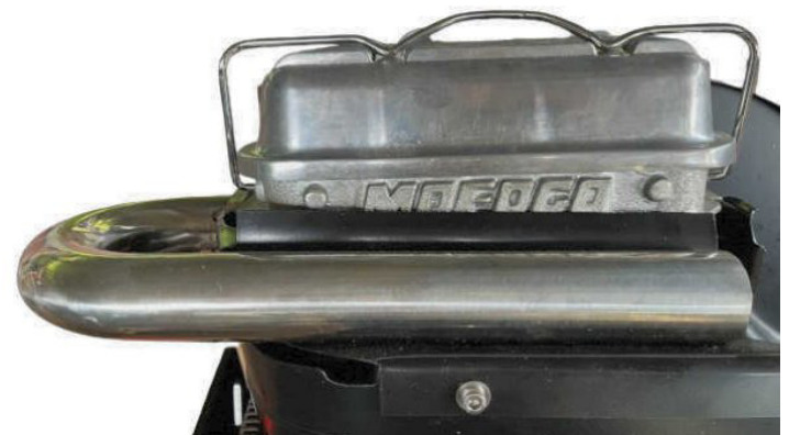
Pulley tin showing panel beating effort around the oil fitting and the patch above the oil pump. If you look really closely, you can make out the rubber grommet around the dipstick tube.
